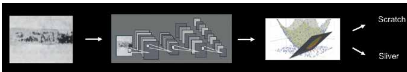
Fig 3: Deep convolutional networks for classification of surface defects
